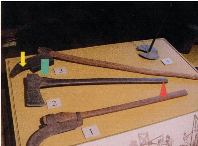
Sledges, axes, and hammers = Third Class Levers
